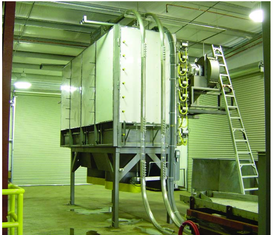
The 18-foot-tall conveying system features a variable-speed drive that allows 2,000 pounds of pecans to be conveyed about every 2 hours.
