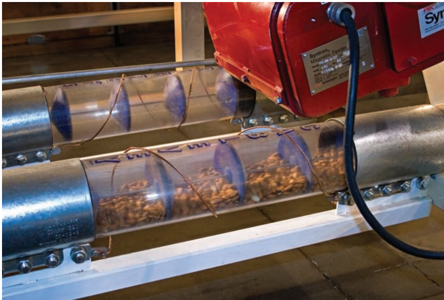
The ultrahigh-molecular-weight plastic discs gently pull the almonds through the conveying tubes.
